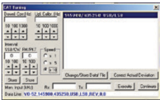
Figure 5 — Click on CAT in the menu bar and set the interval frequency to 0 for both SSB/CW and FM. Also select X10 speed as shown.
